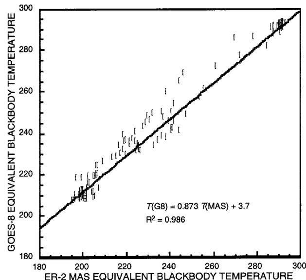
**Figure 4.** Correlation of ER-2 MAS band 45 and GOES-8 channel 4 temperature data during flight leg 2, October 12, 1995.
