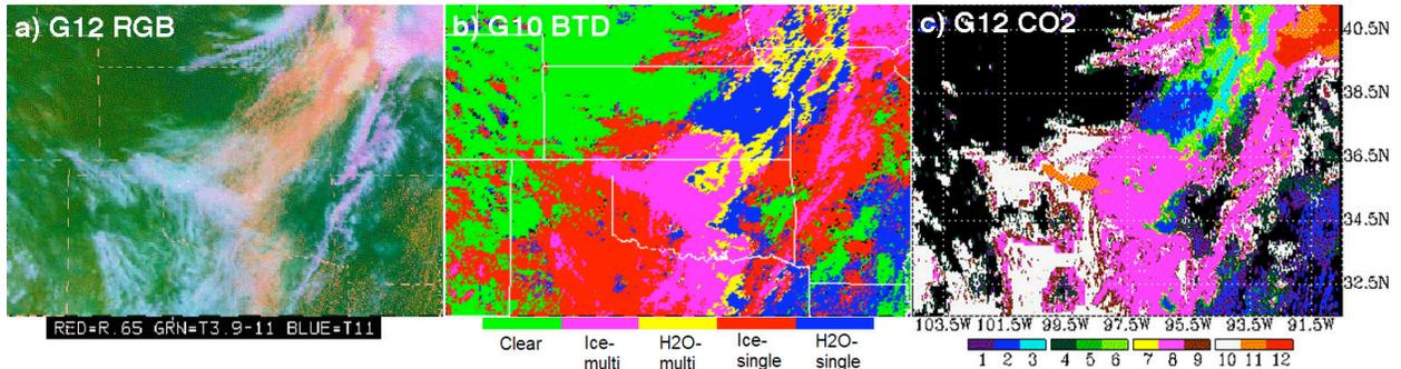
Fig. 1. Cloud layering from GOES imagery, 1915 UTC, 5 May 2005. (b) Phase is given for single-layer retrieval. (c) 1-3: low single-layer, 4-5: mid single-layer, 7-9: multi-layer, 10-12: high single-layer
